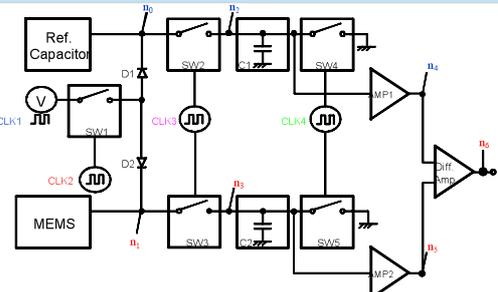
Concept of Switched Capacitor Circuit
