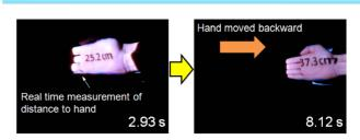
We proposed and built an interactive display based on laser scanning display and laser range finder that is able to input commands by hand gestures.
