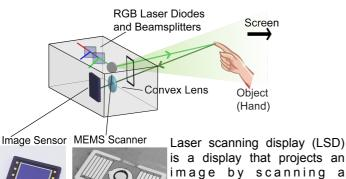
Laser scanning display (LSD) is a display that projects an image by scanning a modulated laser beam spot vertically and horizontally on the screen.
