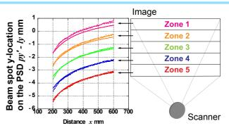
Y-axis shows the Beam spot location on the PSD calculated from the PSD output. Measurement is synchronized with the scanner movement so distance of multiple area can be measured. If the area gets small noise increases. Dots are measurement and lines are calculation result and as shown in figure above dots were on the lines.
